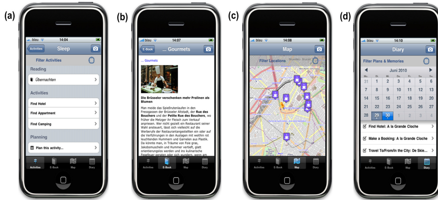
Fig. 9. iPhone screenshots. (a) Activities Mode: the task-based UI allowing for content provision and planning (b) EBook Mode: the content view offering structured and unstructured content (c) Map Mode: the spatial view showing POIs on a full-screen map (d) Diary Mode: the spatial view showing users plans and memories
