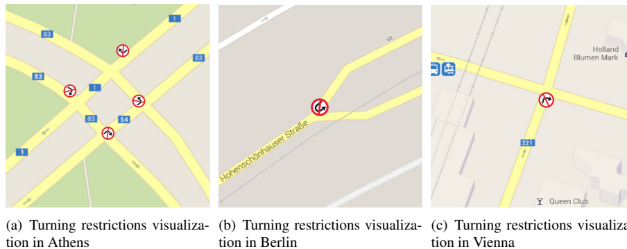
Figure 5: Visualizing turning restriction with QGIS
